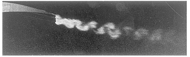
Fig. 9 Smoke-flow visualization, flow from left to right, U_\infty = 10 , \alpha = 0.0 deg.
